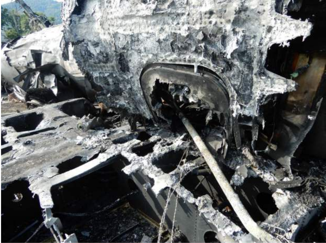
Figure 3: Emergency escape hatch impaled by a metal fence post.
